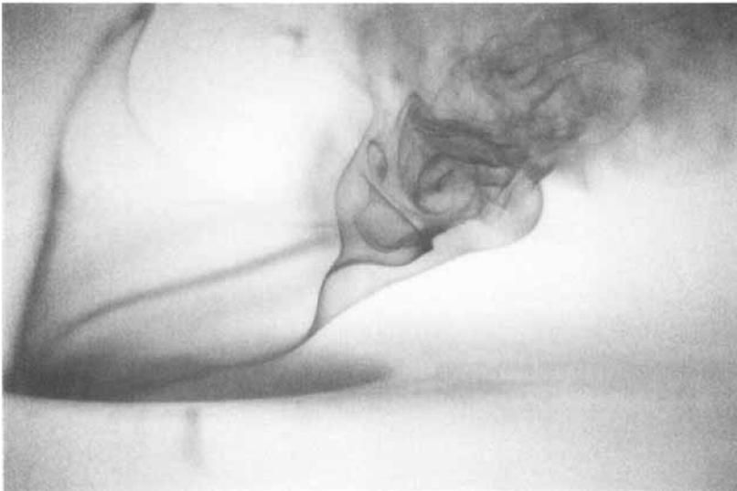
FIGURE 7. Close-up view of vortex breakdown in the CVP at  $Re = 1600$ ,  $R = 4.0$  and  $\delta/D = 0.61$ .
