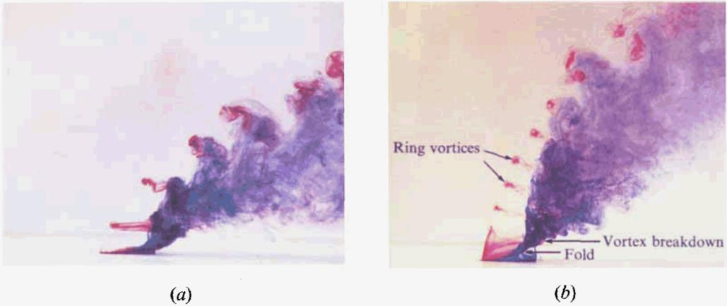
FIGURE 5. Behaviour of the jet shear layer for velocity ratios (a) 2.2 and (b) 4.0 at  $Re = 1600$  and  $\delta/D = 0.61$ . In these photographs, blue dye is injected from the circumferential slot in the pipe and red dye is released from the dye injection port.
